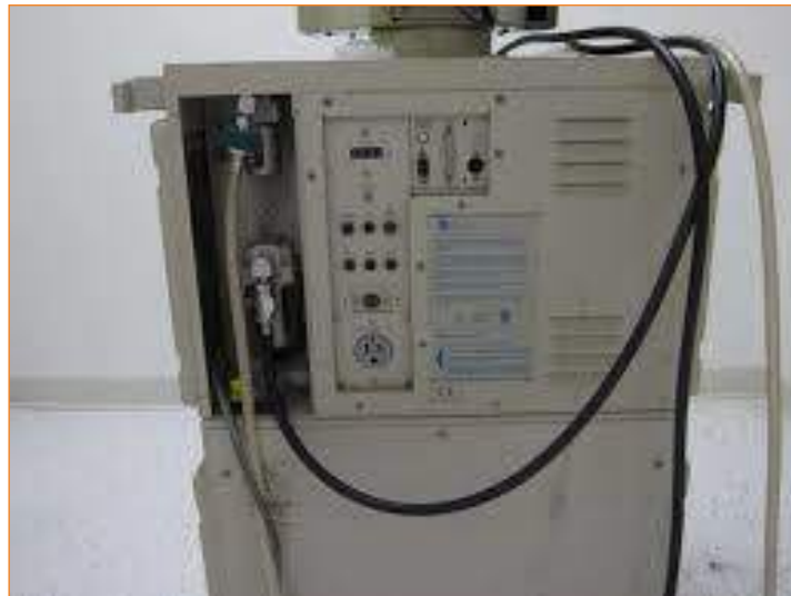
Fig. 4.3.19. Back View of a Ventilator with Oxygen and Air Hose connection
