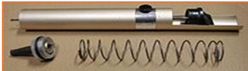
Fig. 1.2.5. Desoldering Pump with the parts opened
