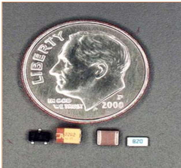
Figure 3.3.1. Showing the small size of SMD Devices-From left to right: SOT-23 bipolar transistor, 2.2 mfd tantalum capacitor, ceramic capacitor, and 82-Ohm resistor. Compare the size concerning a Coin.
