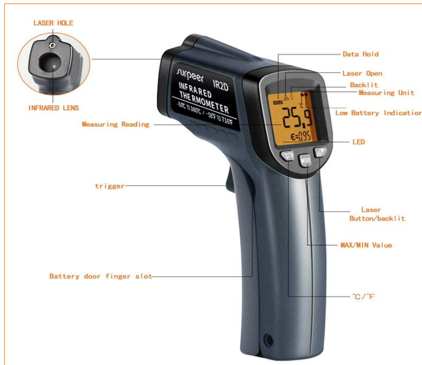
Fig. 4.3.52. A commonly used IR Thermometer to take a contact-less reading of patients.
