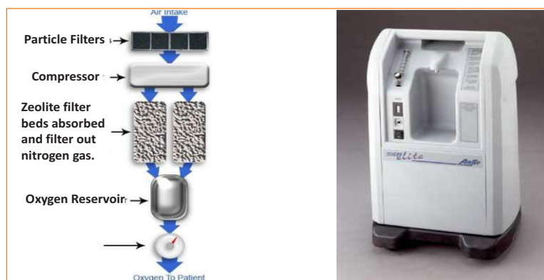
Fig. 4.3.33. Working of Oxygen Concentrator with parts
